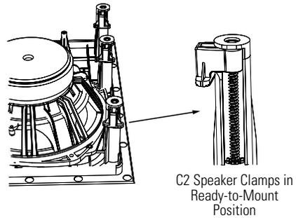
6. Insert the speaker straight into the mounting opening. Tighten the speaker clamp screws on the front of the speaker baffle. The speaker clamps will automatically rotate into position and begin clamping the speaker.
