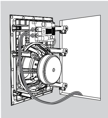
5. Make sure all of the speaker clamps are retracted in their "ready-to-mount" position at the tops of the mount towers, tucked within the mounting opening's border.
