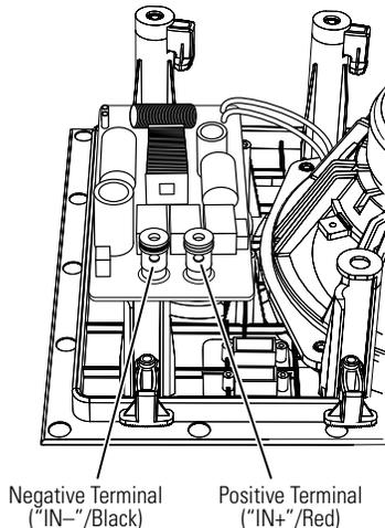
Press down on the top of the terminal to open the hole; insert the bare end of the wire into the hole; and release the terminal to secure the wire.
